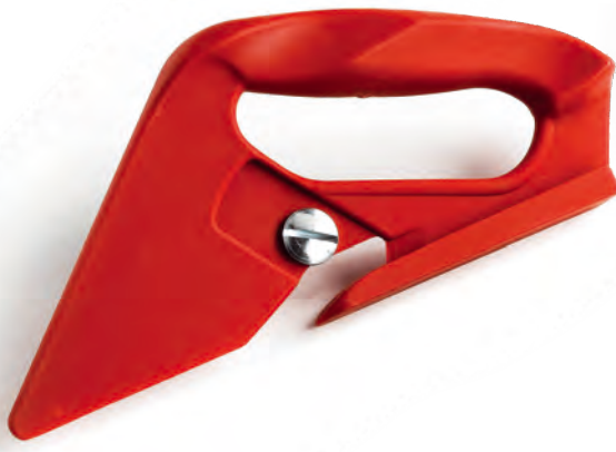
F7550 Combi Carpet Trimmer Extra-long nose separates carpet rows and the spring arm forces material down and towards the cutting blade.
