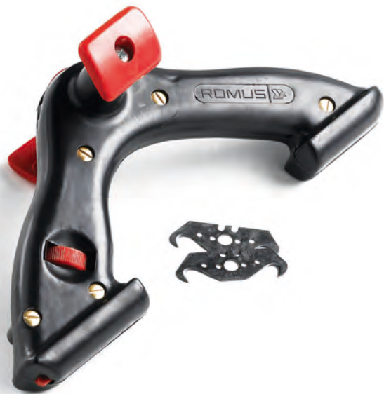
F7553 Hgh Tech Cutter Quick and easy trimming for all types of floorcoverings. Adjustable stops allow the cutter to tilt to a predetermined height depending upon the thickness of the floorcovering.
