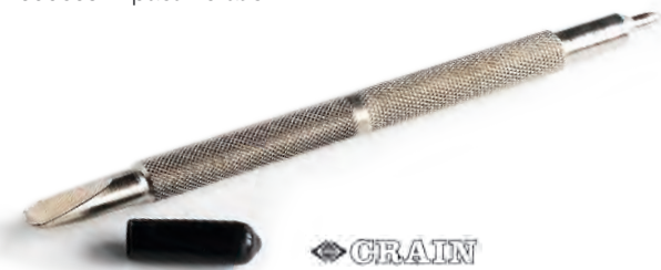
F7035 Row Separator This tool will effectively open and spread rows for reduced shearing of carpet nap by the seam cutter. This double-ended tool has a pointed end for cut pile with a wider conical surface behind the point.
