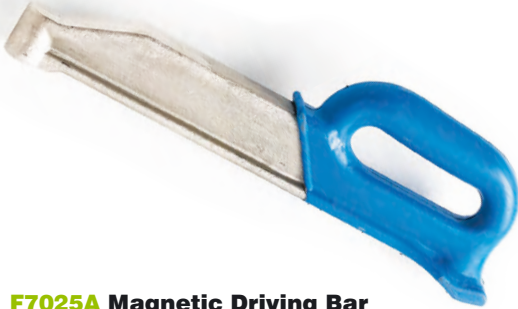
F7025A Magnetic Driving Bar This long-nosed hammering tool extends beneath radiators and other low clearance areas. The hammering tip is magnetised to temporarily hold a nail in position. The forged alloy steel body includes a bonded rubber-like handle that reduces impact vibration.
